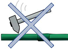
Components of plastic piping system must be protected against damage during transport and installation.
